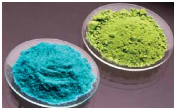
Figure 4.23 Although they are both made of copper and chlorine, copper(I) chloride has a greenish colour, whereas copper(II) chloride has a bluish colour.
